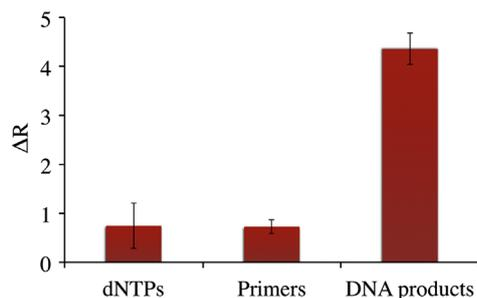
**Fig. 5.** Biosensor response to the individual components of a PCR mixture: dNTPs (0.2 mM each), forward and reverse primers (0.2 μM each) and a purified 35-cycle PCR product. Each response is expressed in terms of the absolute value of the shift in rectification ratio. The symbols and error bars refer to the mean and  $\pm 1$  standard deviation of the values from separate nanopipettes ( $n = 5$ ).
