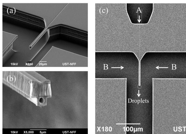
FIG. 2. SEM: (a) isometric view of the flow-focusing geometry with the suspended micronozzle, (b) close-up view of the micronozzle tip revealing the circular opening, and (c) planar view of the microfluidic design with the arrows denoting the flow directions A for discrete phase and B for continuous phase.
