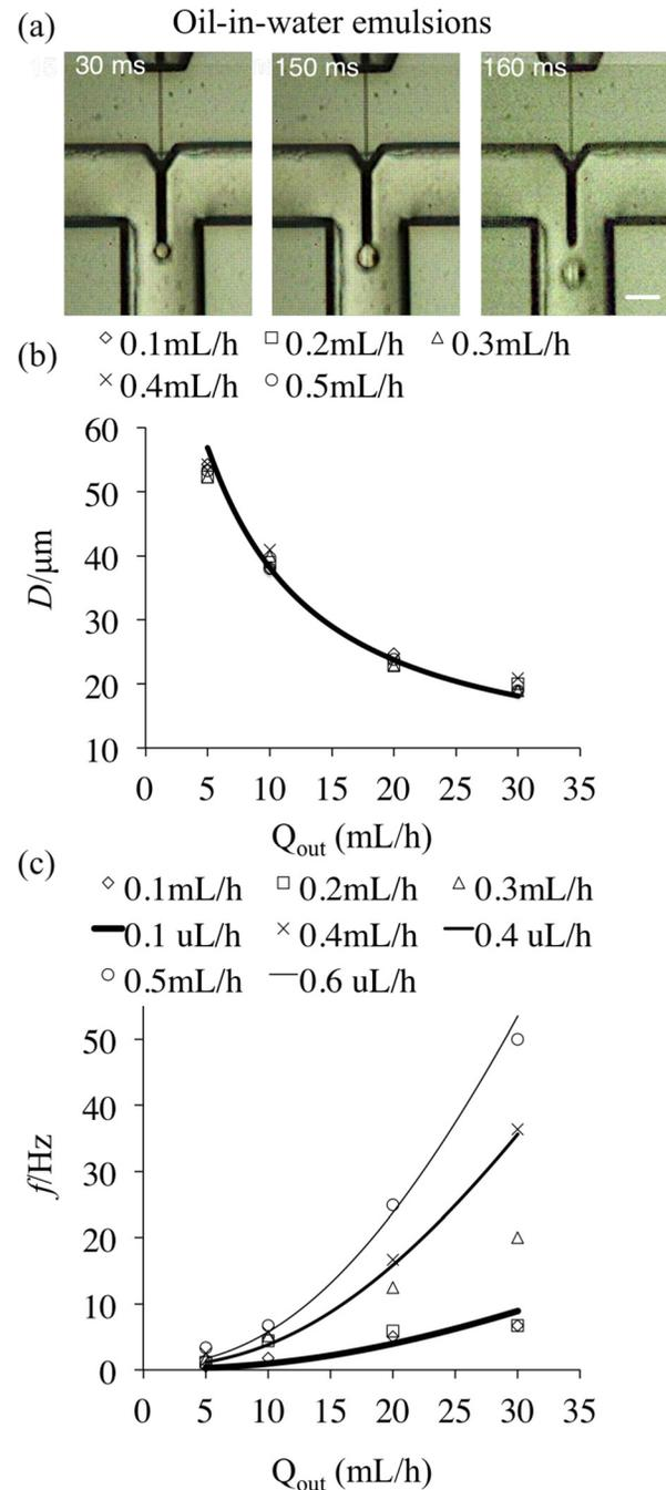
FIG. 4. Oil-in-water emulsions. (a) Time-lapse images showing a single oil droplet forming at the micronozzle tip in a coflow of water. (b) Droplet diameter  $D$  and (c) droplet generation rate  $f$  plotted as a function of water flow rate  $Q_{out}$  for distinct set values of the oil pump  $Q_{set}$  (legend). The solid curves are the respective fittings obtained with  $Ca_{crit} = 0.1$  and for distinct values of  $Q_{in}$  (legend) by Eqs. (5) and (6). Scale:  $50 \mu\text{m}$ .
